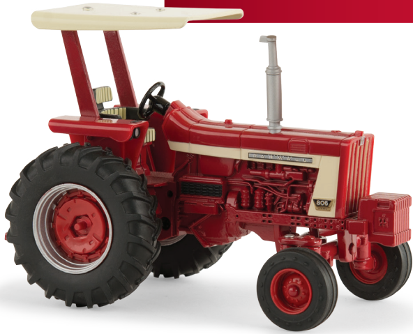
ZFN14999 1:32 Farmall® 806 with ROPS Pack: 3 - Age grade 3+ Die-cast body, front axle, and ROPS frame. Rear hitch attaches to most 1:32 implements.
