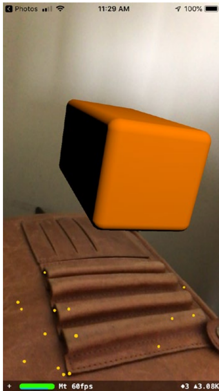
Figure 20-15. An omni light type illuminates the front and top of the orange box
