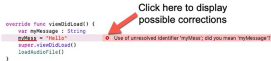
Figure 2-2. Syntax errors often keep a program from running, which allows Xcode to identify the syntax error
